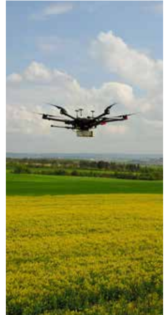
DJI Matrice M600 equipped with RIEGL miniVUX-SYS using RIEGL Integration Kit 600
