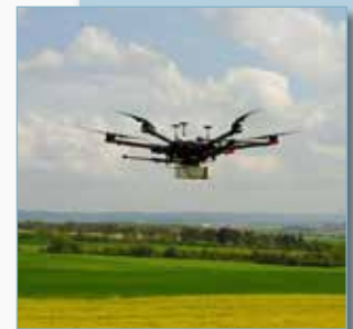
DJI Matrice M600 equipped with RIEGL miniVUX-SYS using RIEGL Integration Kit 600
